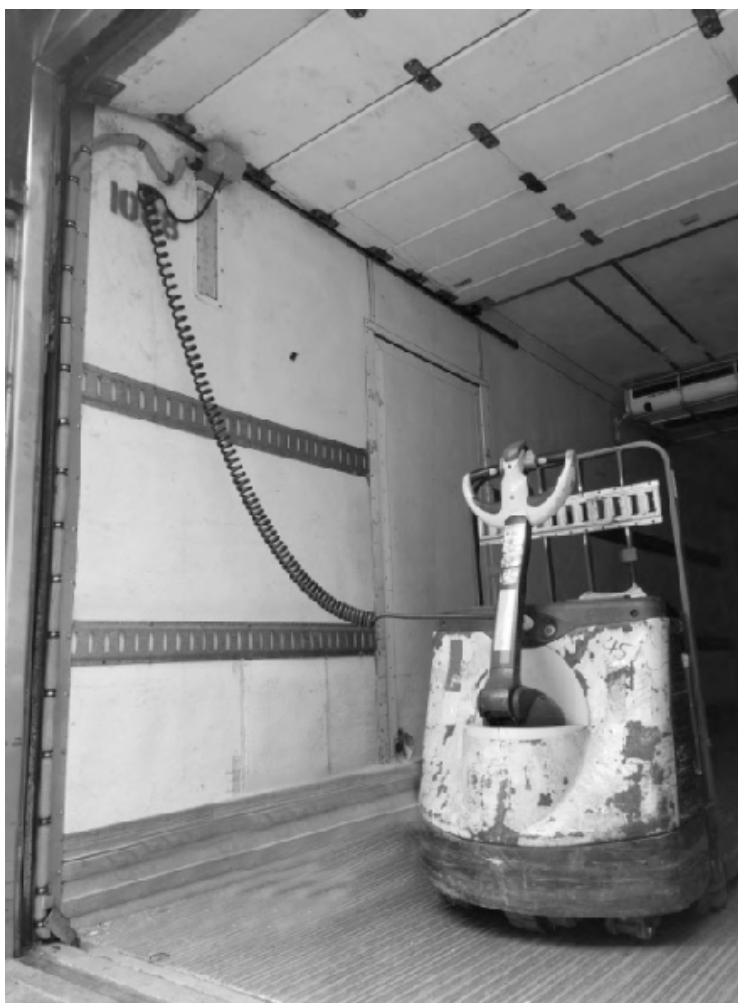
Figure 6. EPJ Shown Connected to GFCI Outlet
